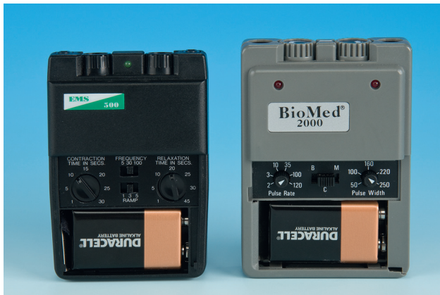
Fig 10-3 A look at the controls will likely indicate what a device can do. A muscle stimulator allows control of the on- and off-time, ramp, and frequency. TENS units often have controls for pulse duration, frequency, and modulation.
