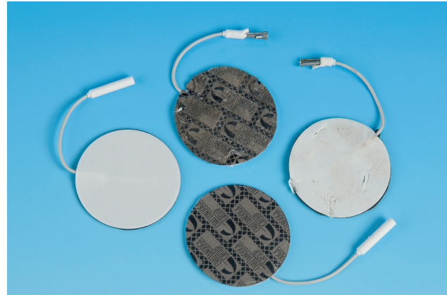
Fig 10 ■ 6 Visual inspection of electrodes prior to and after use is recommended. Breakdown of the connector and conductive surface is common after several uses.
