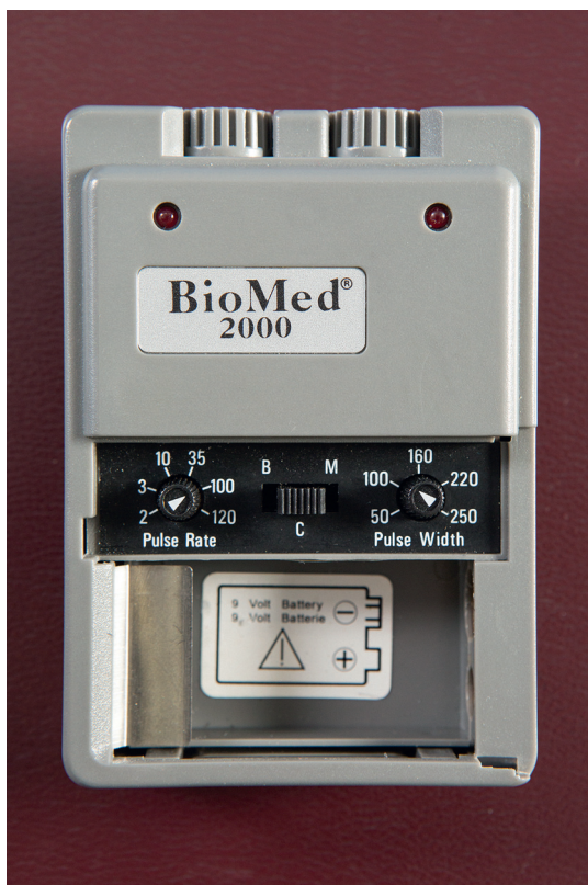
Fig 11 ■ 4 A TENS unit with a slide-switch control for selecting burst (B), continuous (C), or modulated (M) pattern TENS.
