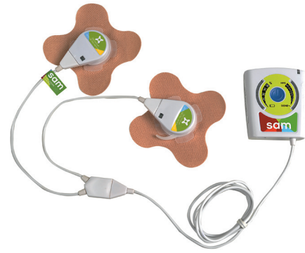
Fig 4 ■ 11 Sustained acoustic medicine (SAM) is a new technology used to provide controlled-release, long-duration US treatment for up to 4 hours daily. (Courtesy of ZetrOZ, Inc., Trumbull, CT.)
