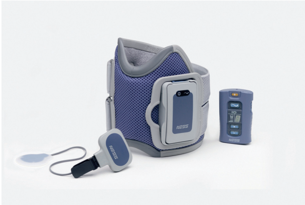
Fig 14 ■ 10 This figure shows, from left to right, the sensor that detects pressure increasing and decreasing beneath the heel, the cuff that contains the electrodes that is wrapped around the patient's proximal tibia/fibula to stimulate dorsiflexion during swing, and the FES controller. (Courtesy © 2009 Bioness, Inc., Valencia, CA)
