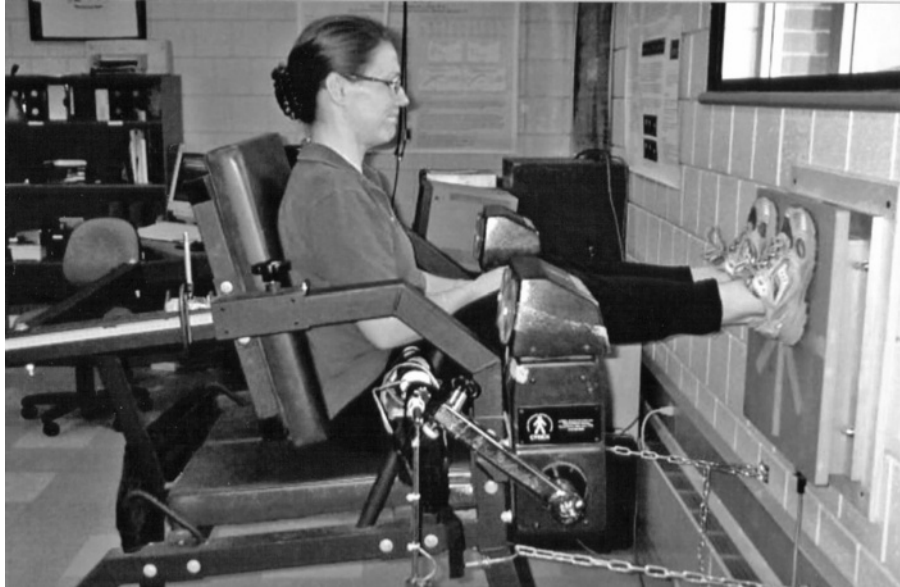
Leg press strength is being measured with a force plate attached to a wall. The force plate is connected to a computer where peak force and rate of force developed are displayed.
