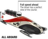
The driver steers the sled; the brakeman slows it after the finish line by moving a rear-mounted handle that lowers a line of metal teeth into the ice.
