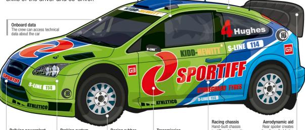
Rallying powerplant All WRC cars incorporate 2-liter, turbocharged engines Braking system Massive ventilated disc brakes provide the stopping power Racing rubber
