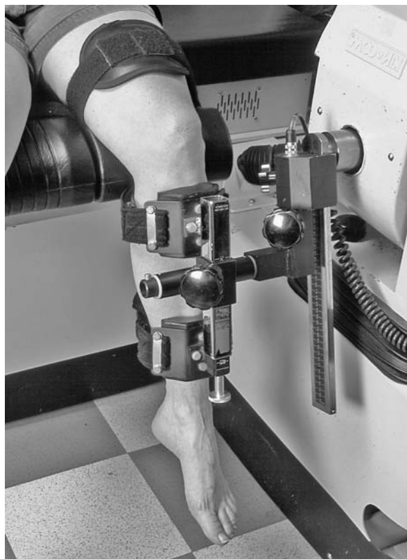
Figure 43.10: A subject exercising the quadriceps femoris on an isokinetic exercise device can use an antishear attachment to protect the ACL.
