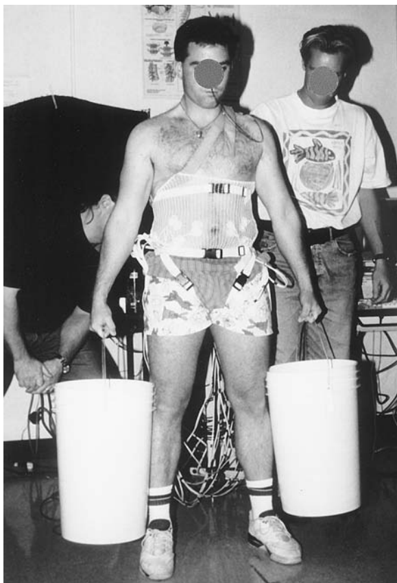
Figure 33.8: Role of active muscle to stabilize the spine. Loading the upright vertebral column (as shown here with the person standing while having weight loaded into baskets in each hand) requires guy wire support from the musculature to prevent buckling. This is an interesting test since muscles, in this posture, are recruited to prevent buckling and not to support moments. In this task, the motor control system appears to choose the abdominal obliques and, to some degree, the quadratus lumborum to provide stability.
