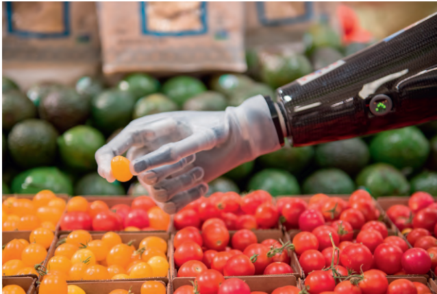
Fig. 30.32 With pattern recognition, the individual's intuitive motor patterns are used to select the desired grasp position and to select operation of the desired component. Here the individual produces a distinct motor pattern to grasp the tomato with index and thumb and a separate motor pattern to rotate the wrist. (© Össur.)
