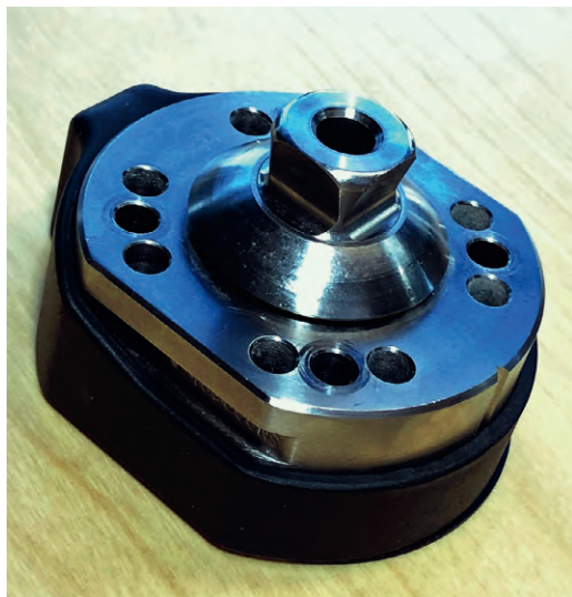
Fig. 23.24 A computerized sensor that can be mounted in-line with other prosthetic components. It can gather kinetic and kinematic gait data as well as socket load in real time. (Reprinted with permission from Orthocare Innovations, Edmonds, WA.)
