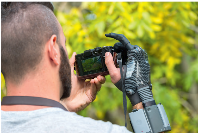
Fig. 30.9 Externally powered active partial-hand prostheses are designed based on the remaining digits and the functional needs of the individual. The multiarticulating iLimb allows for single-digit operation. (© Össur.)
