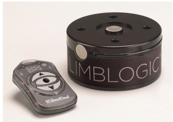
Fig. 23.17 This figure shows a microprocessor-controlled device that draws air out of the socket to maintain the elevated vacuum needed for effective suspension of the prosthesis on the residual limb. Electronic vacuum pumps are reliable and can accurately maintain specified levels of vacuum. (Courtesy of Hanger Clinic, Austin, TX.)
