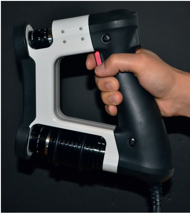
Fig. 23.19 An optical scanner for shape capture. These units allow a mold to be created without having to physically contact the body segment and serve as a method of long-term storage of model shapes. (Photo courtesy Todd DeWees, CPO, Shriners Hospital, Portland, OR.)
