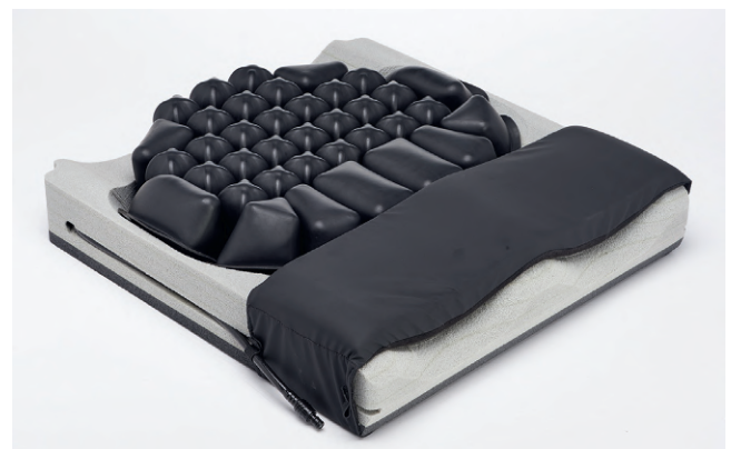
Fig. 16.3 Hybrid cushion includes a contoured base for redistribution of pressures and air-filled bladder to achieve envelopment. (Courtesy Permobil Inc.)
