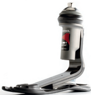
Fig. 21.8 K3 dynamic response foot with vertical shock and torque absorption—OttoBock Triton VS. (Courtesy of Otto Bock Health Care, www.ottobockus.com .)
