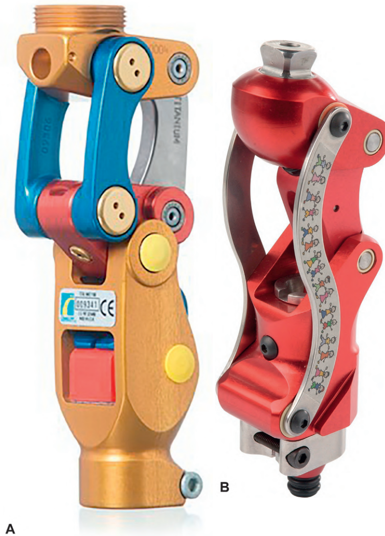
Fig. 29.15 Polycentric knee units used to provide stability and aid in initiation of smooth gait pattern. (A) Total Knee Junior. (B) 3R66 Knee Joint for Children. (A, © Össur. B, Courtesy Otto Bock Orthopedic Industry, Inc., Minneapolis, MN.)
