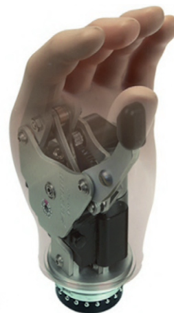
Fig. 30.22 Single degree-of-freedom hand. (A) Three-jaw chuck grasp of steering wheel enhances driving performance. (B) The internal mechanism of the three-jaw chuck hand is visible through the outer structure. The motor controls movement of the index and middle fingers, while the fourth and fifth digits follow. (A, Courtesy Advanced Arm Dynamics. B, Courtesy Steeper Group.)
