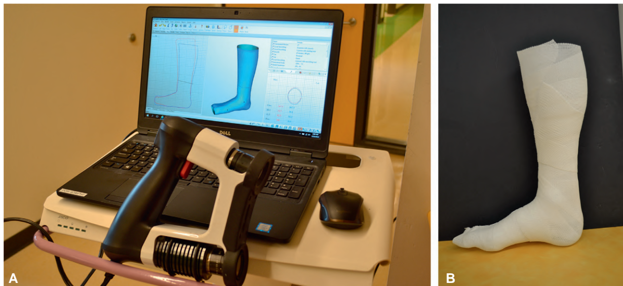
Fig. 6.7 Examples of computer-aided design/computer-aided manufacture data acquisition systems. A digital model of the residual limb (A) can be captured by a laptop computer, appropriate signal processor components, and a handheld digitizer (VORUM—Spectra 3D Prosthetics and Orthotics Scanner, Vancouver, BC). Laser digitization (B) can be used to capture accurately the contours of a conventional negative impression of a residual limb. (Courtesy Shriners Hospital for Children Portland.)
