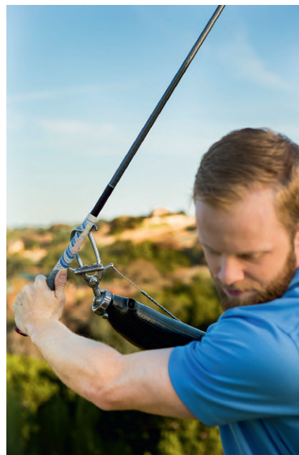
Fig. 30.16 Mobility of the wrist joint reduces compensatory motions in the proximal joints, permitting movement that is more natural and ergonomic. The position on the terminal device with the Robo wrist is adjusted by rotating the base of the wrist unit. (Courtesy of Otto Bock Health Care, www.ottobockus.com .)
