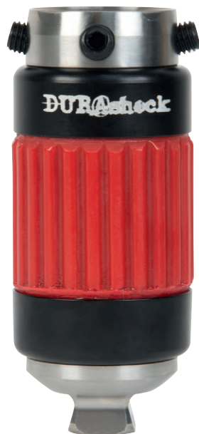
Fig. 23.26 A shock-reducing pylon is mounted directly under the socket to attenuate torque and shock that is transferred from the ground to the limb. It replaces all or part of the pylon, depending on available clearance. (Image provided by Fillauer.)
