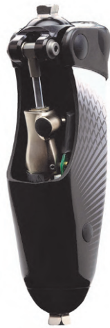
Fig. 27.1 Orion: a pneumatic microprocessor knee unit with stance and swing-phase control. (Courtesy of Blatchford, blatchford.co.uk )
