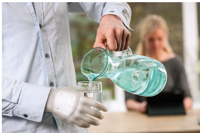
Fig. 30.28 The Michelangelo hand incorporates a wrist that allows ulnar deviation for ergonomically correct positions. (Courtesy of Otto Bock Health Care, www.ottobockus.com .)
