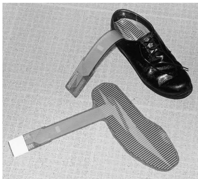
Fig. 5.11 An in-shoe pressure-sensing array can help identify areas of high pressure concentration. This information assists in the design of an orthosis to modify pressure dynamics during the stance phase of gait.
