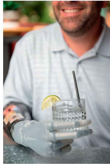
Fig. 30.24 Multiarticulating hands are also called “compliant hands” because they comply to the shape of the object being grasped. Grasping the object with greater surface area provides a secure hold on the object. (© Össur.)
