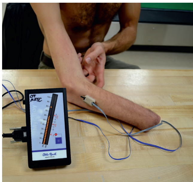
Fig. 31.7 A Myoboy system with surface electrodes is used to locate potential myosites and provide biofeedback to help clients master the types of contractions necessary to control actions of a myoelectric prosthesis. (Courtesy of Otto Bock Health Care, www.ottobockus.com .)
