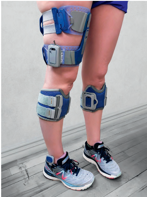
Fig. 9.11 The Bioness L300 System, as an example of a wearable functional electrical stimulation unit, is used to trigger muscle contraction during appropriate points in the gait cycle. The L300 system (photo R) triggers dorsiflexion during swing phase. The L300+ system (photo L) incorporates a thigh component that can stimulate the knee flexors or extensors during swing and/or stance phase to assist with stance stability or swing limb advancement.
